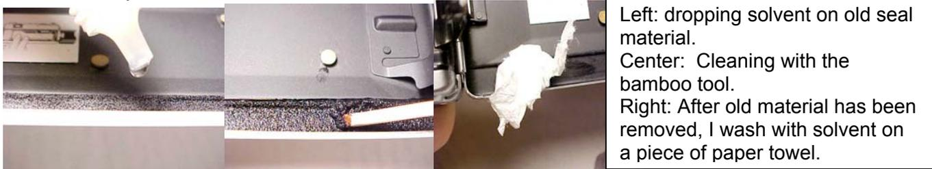
After you clean the old seal from the film door, you'll need to also clean the old seal off the latch end. This is done the same way. This area is cramped, and you'll have to work carefully in here.
