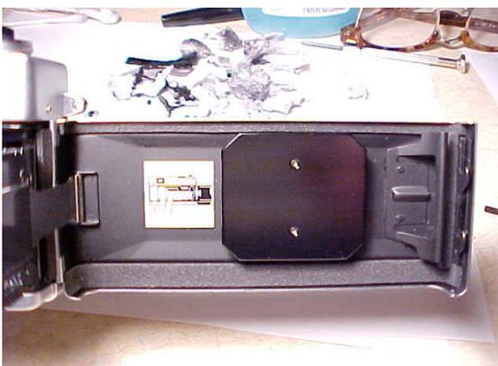
To the left is the way your new seal should look—neat and professionally done. You may replace the pressure plate by reversing the steps to remove it. To the right is a view of the latch end all re-sealed. There is a surprise here, and we'll talk about this next...
