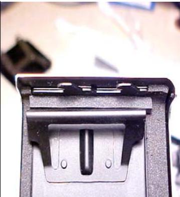
The last piece of seal material you have to install is used for the latch end seal. This is cut from 3mm thick self-adhesive foam, and it is 2mm x 45mm) When you cleaned the seal material off of this area, you probably noticed there were two flanges (tabs) underneath the old seal. Let's take a look at those, because this is important.
