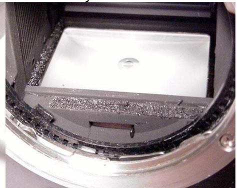
In the first image above, you can see the old damper pad. It may still look ok, but it probably isn't. In the middle image, you can see how I use the tip of a hobby knife (like an X-Acto knife) to carefully remove the old pad. Tilt the camera so that anything you remove falls away from the focus screen and out the lens opening. In the final image, you see how things look after I have made the first pass with the hobby knife. I have removed most of the old pad. Now, look below:
