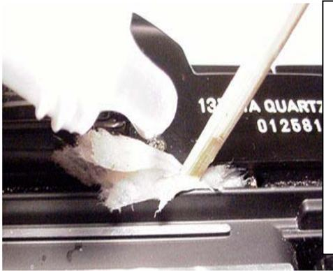
Left: Using a bit of paper towel and solvent, I begin to clean the long thin body slots using the thin end of my bamboo tool. Be careful not to push old material into the film counter reset pin. You can see it beneath the letters "MA" on the top plate. Right: I begin to install the "Seal Strip."
