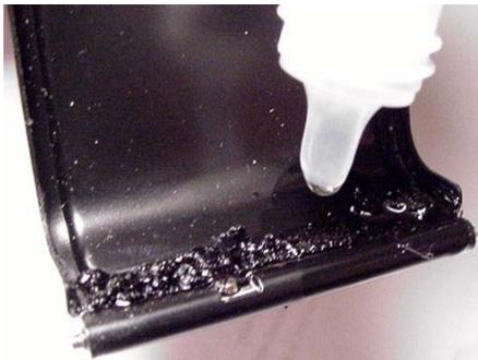
Left: you can see I am dripping solvent on the old foam. I will use my bamboo tool and bits of paper napkin or towel to clean the old foam and adhesive from the hinge end and the latch end. To the right, you can see how the door will look when it is clean.
