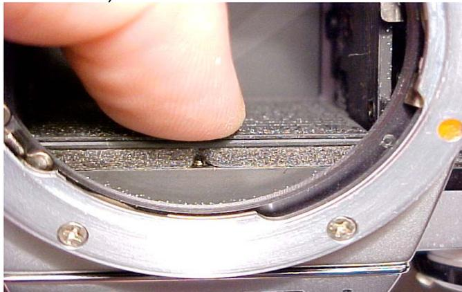
Simply lift the mirror up gently to meet the newly installed damper pad and press against it. Easy? Yes it is, and you will also provide uniform pressure so that your pad will be installed correctly, just like a pro would do it. Some people tell me they worry about replacing the damper pad, but that wasn't so bad, was it?
