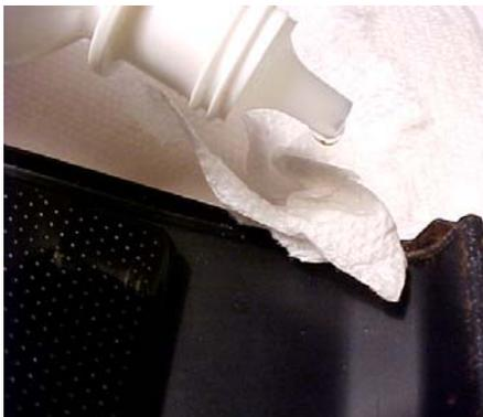
Left: you can see I am cleaning the edges of the film door with a piece of paper towel and solvent. It is important to do this, because you do not want the old foam to ruin your new seals. To the right you see I have installed the new hinge end seal piece. Lick the adhesive side to give more time to position.
