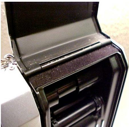
Left: I've replaced the hinge end seal with 1mm thick fabric seal material cut 49mm x 6.5mm. Right: I've replaced the latch end seal with 1.6mm thick fabric cut 46mm x 6mm. This is wider than original, but it will be a vast improvement. Remember: lick the adhesive side to delay adhesion and give you time to position the pieces accurately.
