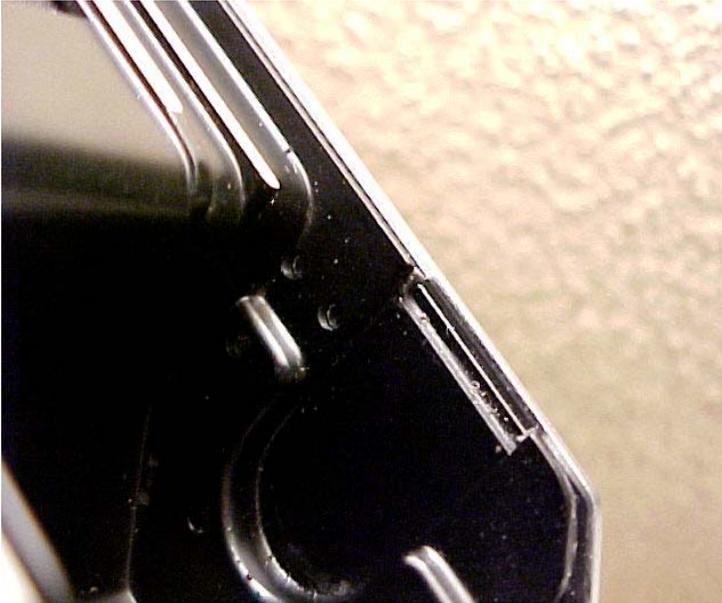
**Important note:** To the left, you will see a cutout on the bottom rail slot of the body. Stop the seal foam at the start of this cutout and resume it on the other side. Failing to do this will cause the film canister to catch the seal piece and pull it out when the roll is changed.
