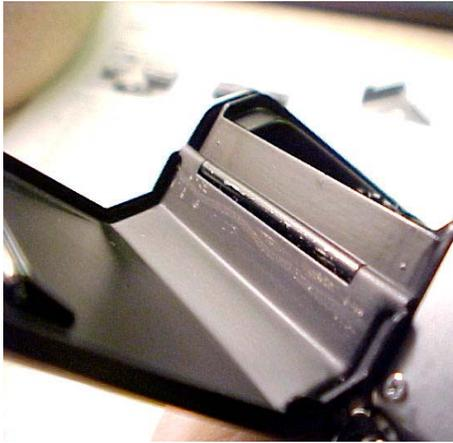
Left—the hinge area nicely cleaned. As you can see, the paint on my film door was degraded by the old foam goop. This is normal, and you can repaint this if desired. To the right, the latch end area cleaned. You'll notice the old seal foam has caused a bit of paint loss there, also. Again, not the end of the world, but you can fix if you wish.
