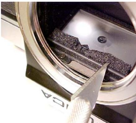
Top left: I use an X-Acto style hobby knife to remove the old damper pad. Be careful, work under a good light, and tilt the camera so that the loose foam you remove will fall out the lens opening and not on the screen.
