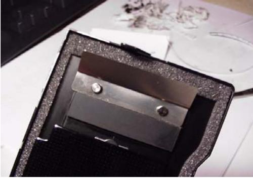
For the latch end seal, cut a piece of 1.5mm self-adhesive foam 6mm wide by 45mm long. Remove the backing paper, lick the piece well and fit between the side pieces you've installed. While wet, position as needed and let it dry. In 20 or 30 minutes, you can press it down for the final fit.
