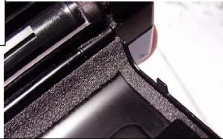
The side door seal installed, as shown above (right). Please lick or wet before installing to allow time to adjust for fit.
