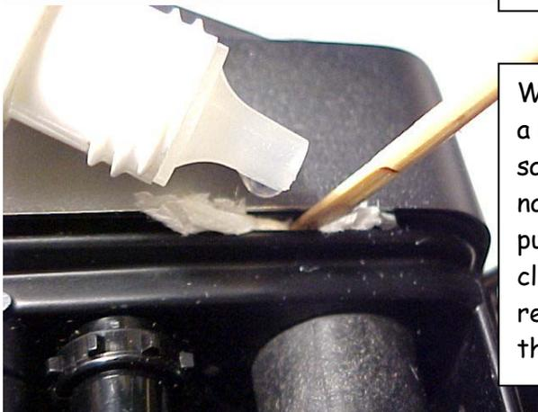
We'll start by cleaning out the film door slots. Press a bit of paper napkin or towel into the slot and saturate it with a solvent like denatured alcohol or naphtha. Using the thin end of your bamboo tool, push this bit of napkin through the slot until it is clean. Be careful to avoid the film frame counter reset lever. It is about 1 inch from the left end in the top slot. Clean both top and bottom slots.
