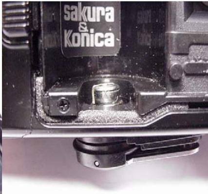
For the seal at the bottom of the film canister cutout, I'd use a thin piece of 1.5mm thick self-adhesive foam cut about 1.5mm wide. **Lick** the piece well and slip it into the slot. Once your saliva has dried, you can press it down for a final fit. The non-adhesive strip would be disturbed by the film canister in this case
