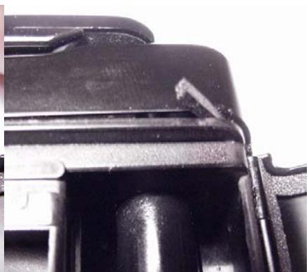
Take a long 2mm piece of non-adhesive seal material and press it into the slot using your fingertip. Use the small end of your bamboo tool to guide it in and press it down, and be sure the skinned (or slick) side faces outward. Start at the hinge end and work toward the film frame counter. Don't worry that there is no adhesive.
