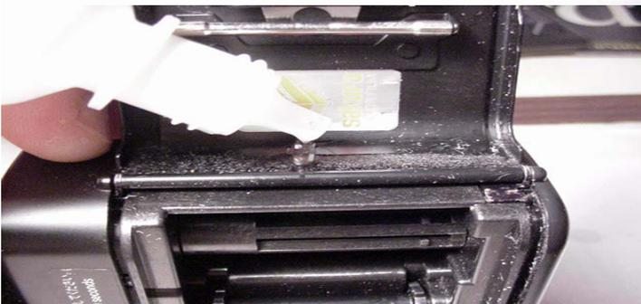
As before, I apply solvent to all the old seal, remove and clean well. Be careful not to scratch the paint under the old seal. Unfortunately, the person who re-sealed this camera may have used a screwdriver tip to remove the old seal and that can leave scratches.
