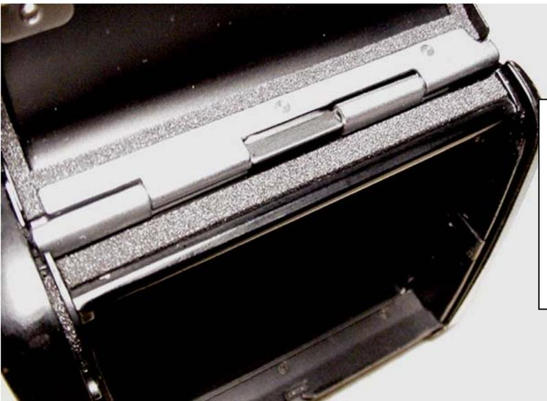
And last, the hinge end seal. This is a simple seal which is made with 1.5mm thick foam cut 76mm long x 4mm wide. Installing it is just a matter of licking the adhesive side and positioning as needed. After this seal (and all the others) are dry, press gently down for the final installation.
