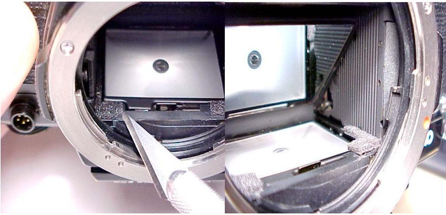
Left: the damper pad in an Olympus OM-1. It is an "L" shaped pad of 1.5mm foam. I carefully remove with the knife blade.
