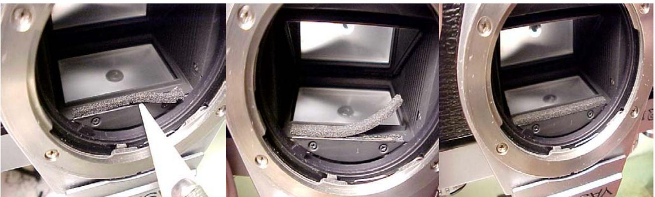
Yashica FR II. Left, I remove the old pad. Notice the ledge behind it. Center, I replace with a new 1.5mm open-celled pad. Right, the job is finished, and the camera is like new again.
