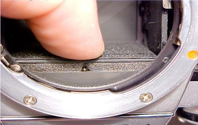
In this Pentax ME, you can see a little cutout for the focus screen adjustment screw. I've done this to make sure the damper pad sits straight across the top...otherwise, it would be like a rock under your mattress. To make such a cut, simply use a small pair of scissors and nick a "V" into the center of the pad.
