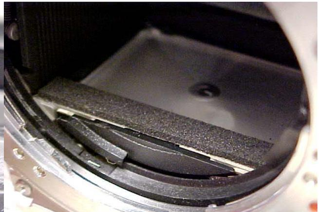
Above, you see the damper pad in an Olympus OM-10. Please note it is different. The original pad was a 1.5mm "sandwich" pad, but it isn't available any longer. The best thing we can do is to carefully remove it and replace with a 1.5mm self-adhesive open celled pad, as I've done in the frame to the right.
