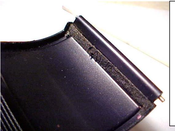
←As you look at your film door, you will see the old seal foam at the end. Our first job will be to remove it. Using solvent and the wide end of your bamboo tool (or similar wood scraper), carefully remove the old material as shown to your right and described below.→
