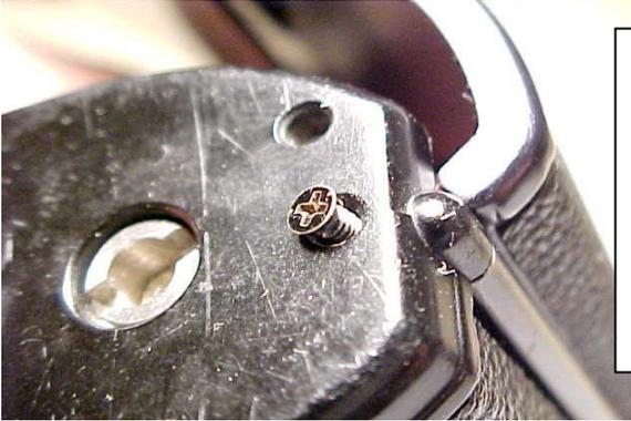
As you look at the hinge end of the bottom plate, you'll see a small Phillips head screw. Loosen it, or remove it, and lift up gently on this end of the bottom. You'll be able to remove the film door, and this is what I want you to do. Once the film door has been removed, replace the Phillips head screw and tighten it...we don't want to risk losing it. Removing your film door will make it much easier to clean and replace the old seal material.
