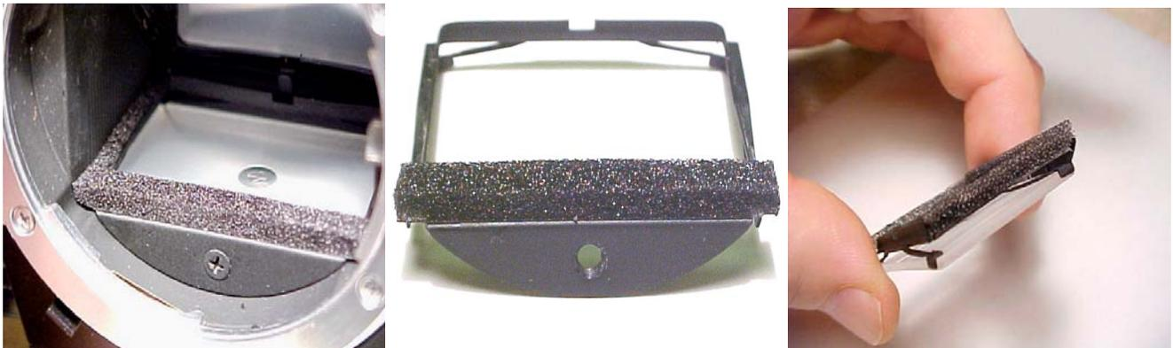
There are three pictures above. The first one shows the mirror damper after it has been re-done. I did not show the "before" picture, because in this camera, the damper was almost all gone. The middle picture shows the damper frame without the focus screen (with the front piece of foam
