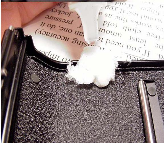
Left: I use a bit of paper towel and solvent to clean the edges of the film door. These will have old sticky foam on them, and you don't want this to foul or stick to your new foam. This is actually an image of me cleaning the film door of an F2 model, however this procedure is the same for all cameras.
