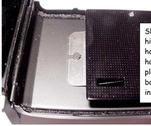
Slide the pressure plate back (moving away from the hinge end) until the tab is clear of the small button holder. Then you can "click" it away from the button holder on the other side. Please note the pressure plate must be installed with the cutout at the bottom of the film door. The film tractor wheel fits into it. Set the pressure plate aside for now.
