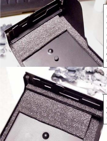
While I am at it, I will also install the small pad which sits above the film canister retaining pad. This is also made from 1.5mm thick foam, and it measures 49mm x 2.5mm. You can <u>lick</u> this piece before you install it, also. Doing this will make your work much easier and more accurate. (now you see the film door and seal both appear to be straight again.)
