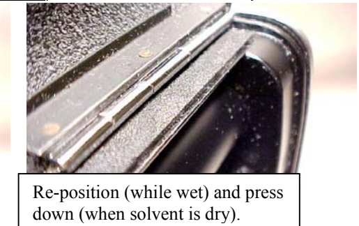
Moisten completely with solvent* and let sit for 1 minute or more. ⌚
