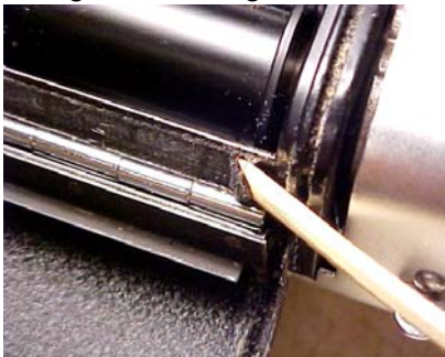
Moisten completely with solvent* and let sit for 1 minute or more. ⌚
