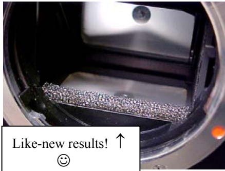
Use the edge or tip of a razor blade to pick away the backing paper ↑
