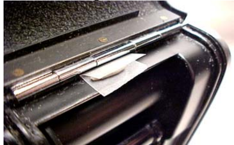
Seal material chosen should be slightly thicker than this. 1mm in this case.
