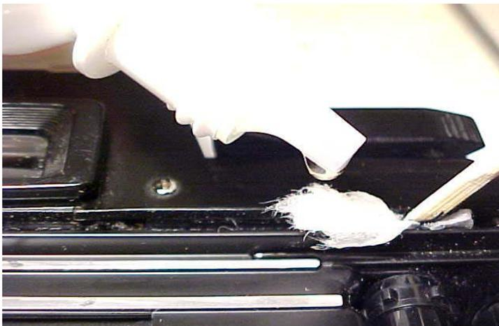
First, run a toothpick with the end broken off or the narrow end of your bamboo tool through the slot to remove the gunk. Repeat if needed, working away from the frame counter reset lever. Be careful not to push old seal material into the frame counter reset area. Then run a small piece of paper towel with a little solvent on it through the slot to finish cleaning it. You may need to do this several times to get the slot fully cleaned.
