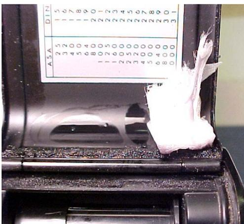
Left, cleaning the hinge seal area with a piece of paper towel soaked in solvent. To the right, I'm doing the same thing to the film door edges. There will be old sticky material left here, and I don't want it to foul my new seal strips. You may also wipe the film pressure plate with solvent to clean it.
