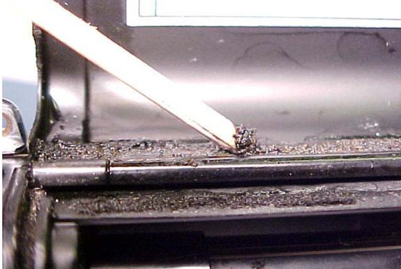
Pretty unimaginative work, but you need to be careful not to scratch the paint. You can see old seal material stuck to the film door and the camera body. In this case, I'm going to replace the seal on the film door, as that is clearly where it was originally located. I'm going to use the 1.5mm open-celled foam, and the strip I will cut is 3.5mm wide x 52mm long. After I have removed as much as possible with the bamboo tool, I will use a piece of paper towel soaked in solvent to finish cleaning.
