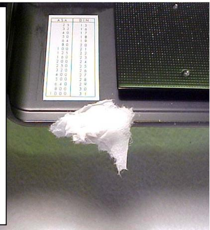
Now we're going to clean out the rail slots on the camera body and replace those seals. Here's how:
