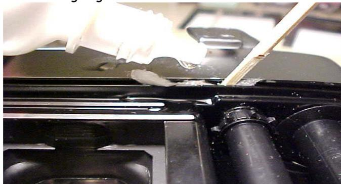
First, run a toothpick with the end broken off or the narrow end of your bamboo tool through the slot to remove the gunk. Repeat if needed, working away from the frame counter reset lever. Don't push old seal material into the frame counter reset area. Then run a small piece of paper towel with a little solvent on it through the slot to finish cleaning. (as shown)
