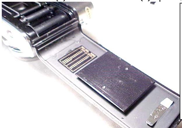
Beneath the top plate, you will see a long thin rail slot. There is a corresponding slot at the bottom. In the top slot, you will see the frame counter reset lever about 1 inch from the right side. There will be a seal at the hinge end, too. It will be on the camera body. This is the basic light seal design used successfully by makers of many models of cameras from the 1950s to present day. It is simple, and it works very well.
