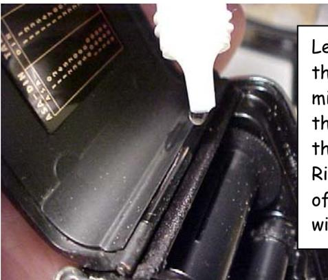
Left: drop some solvent on the old seal. Let it soak a minute or so—don't forget the seal piece at the top of the door.
